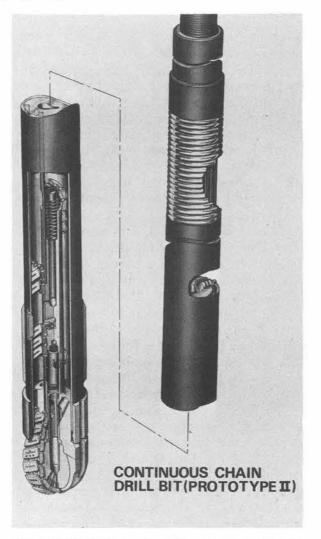
THE CHAIN of the chain drill bit is, in fact, the drill bit; diamond cutters are mounted on the outside surfaces of the individual links. Five such links constitute one drill bit, and the continuous chain may possess up to 15 such bits.
